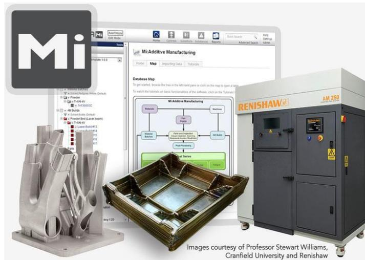
This materials information management system is based on GRANTA MI™, the world's leading materials information management system for engineering enterprises. GRANTA MI has specialist data structures for managing the complexities of materials data. It is possible to configure these structures (the so-called 'schema') to the specific requirements of the user organization or project. Within AMAZE, the Granta team worked closely with the project
