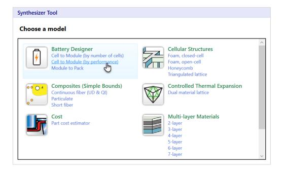
This tool draws on the <u>Battery Cells data table</u> and calculates the estimated electrical and thermal outputs of user-defined cell configurations in multi-cell battery modules and multi-cell/module battery packs. Modules can be specified by either cell configuration or performance requirements, and Ragone charts plotted in GRANTA Selector using the Chart Stage.
