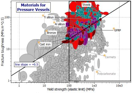
Figure 5-2. A chart of fracture toughness  $K_{IC}$  against elastic limit  $\sigma_y$ , using the generic record subset, showing the indices M2, and M3 = 100 MPa.
