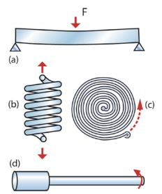
Figure 4-1. Springs have many shapes, but all perform the same function: that of storing elastic energy.
