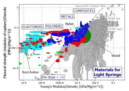
Figure 4-4. A chart of  $\sigma_{MOR}/\rho$  against E/ $\rho$ . The diagonal line is a contour of M<sub>2</sub>.
