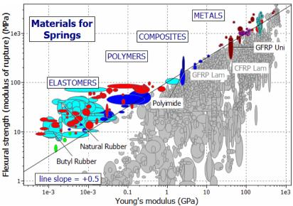
Figure 4-2. A chart of the modulus of rupture,  $\sigma_{MOR}$ , against Young's modulus, E. The diagonal line shows  $M_1$ .
