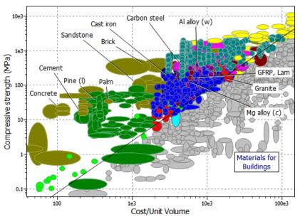
Figure 3-3. The compressive strength,  $\sigma c$ , plotted against cost per unit volume,  $C_m \rho$ , using the 'All bulk materials' record subset
