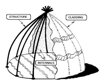
*Figure 3-1.* The materials of a building perform three broad functions. The frame gives mechanical support, the cladding excludes the environment, and the internal surfacing controls heat, light, and sound.
