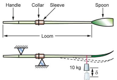
Figure 2-1 Oars are designed on stiffness, measured in the way shown in the lower figure; and they must be light
