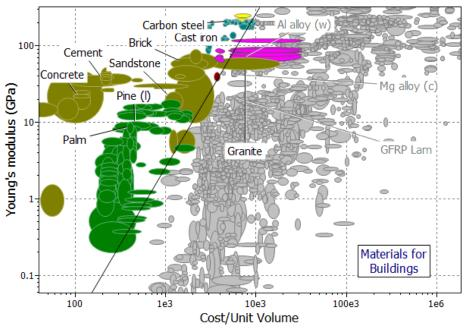
Figure 3-2. The modulus, E, plotted against cost per unit volume, Cmp, using 'All bulk materials' record subset
