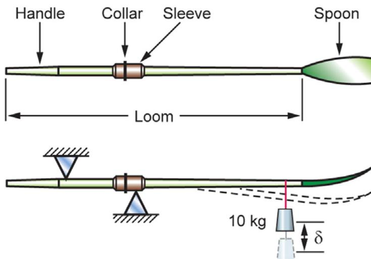
Figure 2-1 Oars are designed on stiffness, measured in the way shown in the lower figure; and they must be light
