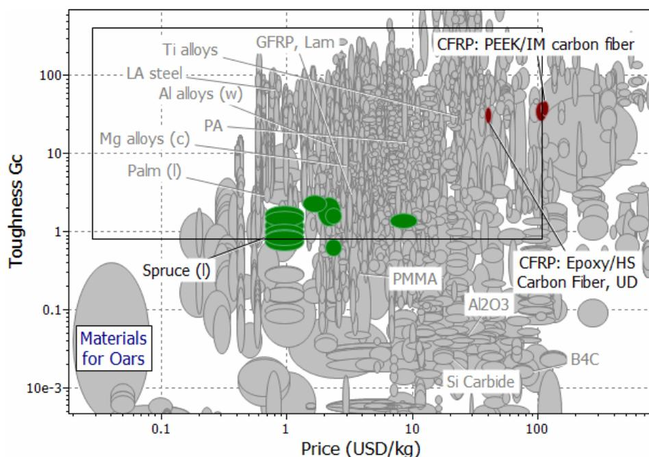
Figure 2-3. An example chart of toughness,  $G_c$ , against cost/kg,  $C_m$ , made at Level 3 of the database. The box isolates materials with  $G_c > 1 \text{ kJ/m}^2$  and  $C_m < 100 \text{ USD/kg}$  (75 GBP/kg).
