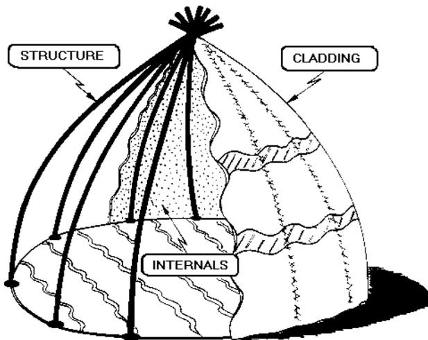
Figure 3-1. The materials of a building perform three broad functions. The frame gives mechanical support, the cladding excludes the environment, and the internal surfacing controls heat, light, and sound.
