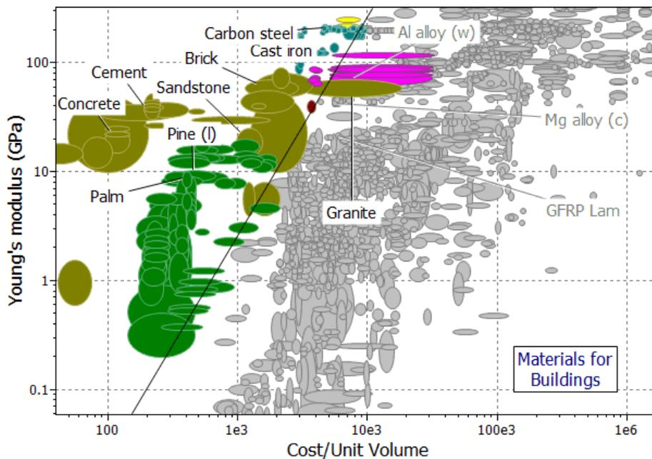
Figure 3-2. The modulus,  $E$ , plotted against cost per unit volume,  $C_m \rho$ , using 'All bulk materials' record subset
