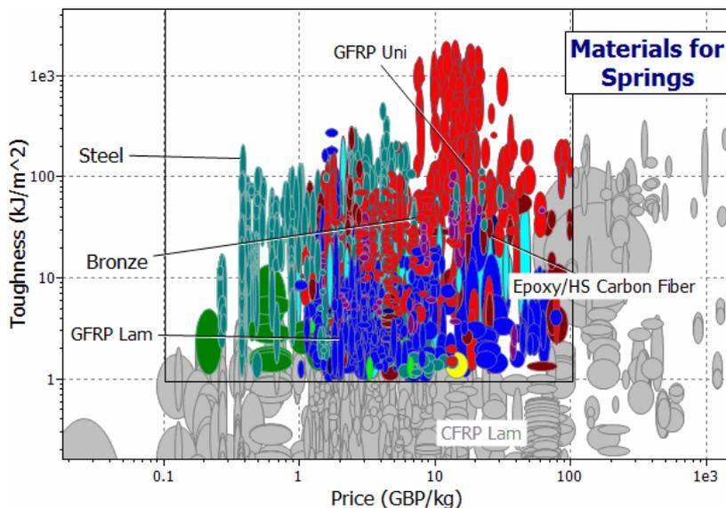
Figure 4-3. A 'protective' chart of the toughness,  $G_c$ , against cost per unit weight,  $C_m$ . The box restricts the selection to materials with  $G_c > 1 \text{ kJ/m}^2$  and  $C_m < 100 \text{ GBP/kg}$ . The currency unit is easily changed in 'Options'.
