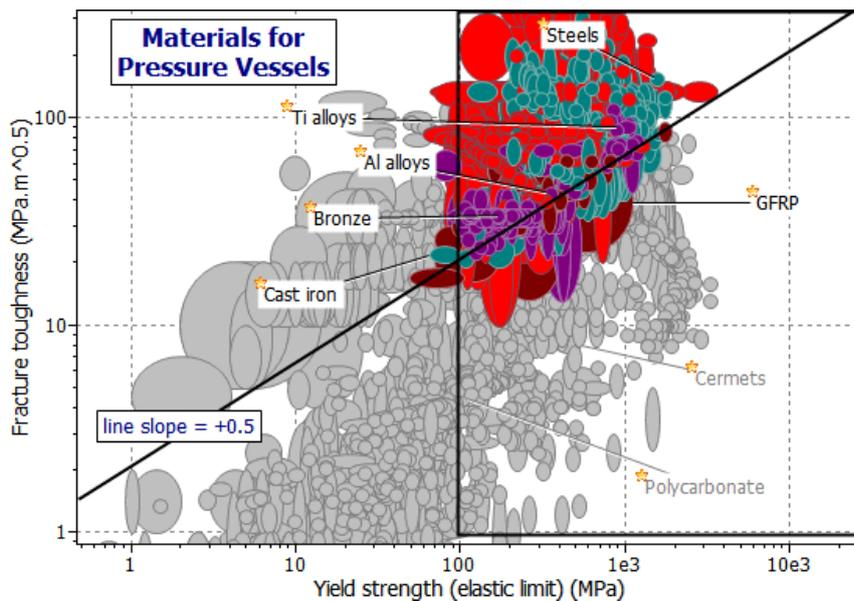
Figure 5-2. A chart of fracture toughness  $K_{Ic}$  against elastic limit  $\sigma_y$ , using the generic record subset, showing the indices  $M_2$ , and  $M_3 = 100 \text{ MPa}$ .
