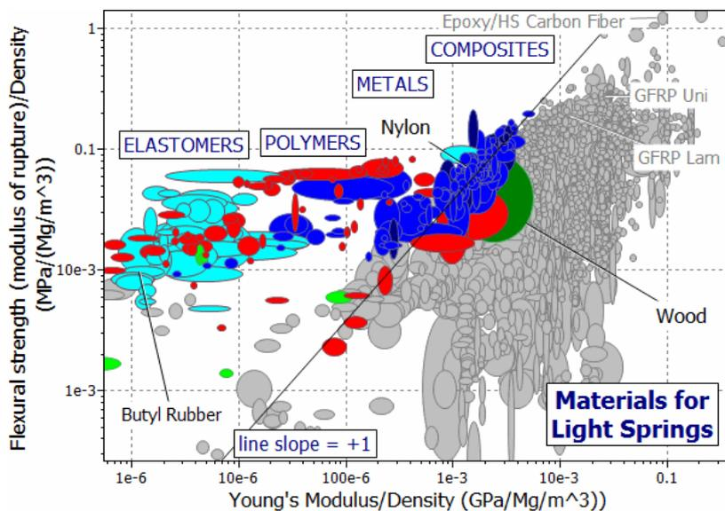
Figure 4-4. A chart of  $\sigma_{MOR}/\rho$  against  $E/\rho$ . The diagonal line is a contour of  $M_2$ .
