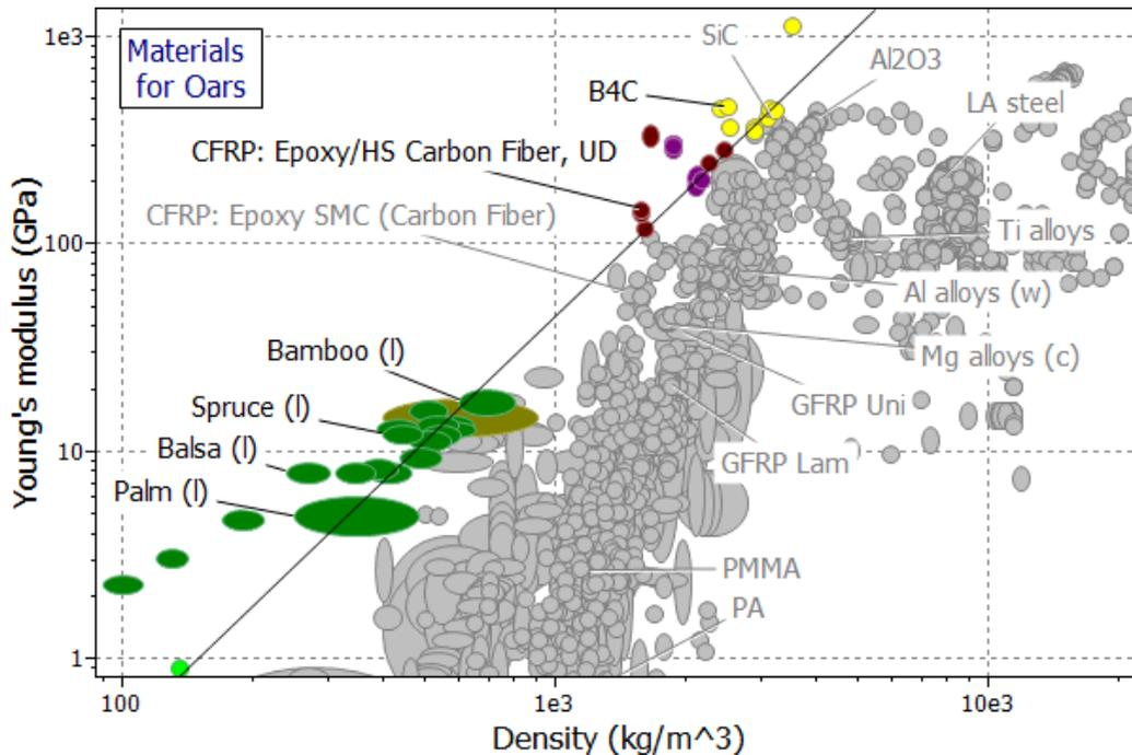
Figure 2-2. A chart of modulus,  $E$ , against density,  $\rho$ . The selection line is placed at  $M_1 = 0.006 \text{ GPa}^{1/2}/(\text{kg/m}^3)$ .
