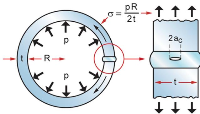
Figure 5-1. A pressure vessel. It must be assumed that flaws pre-exist. The design and choice of material must ensure that they do not propagate.
