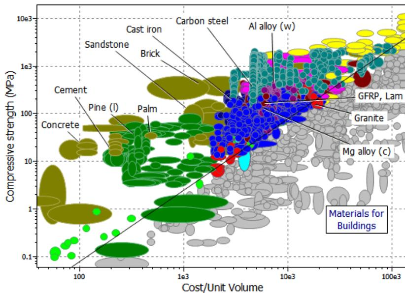
Figure 3-3. The compressive strength,  $\sigma_c$ , plotted against cost per unit volume,  $C_{mp}$ , using the 'All bulk materials' record subset
