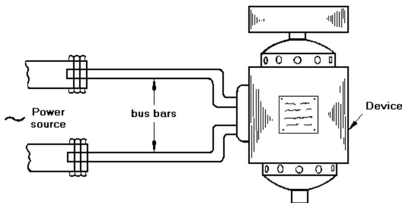
Figure 2-1. Bus bars transmit electrical power from the power source to the device which consumes it.
