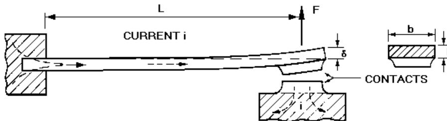
Figure 4-1. A relay arm. It must respond quickly, withstand fatigue loading, and conduct well.
