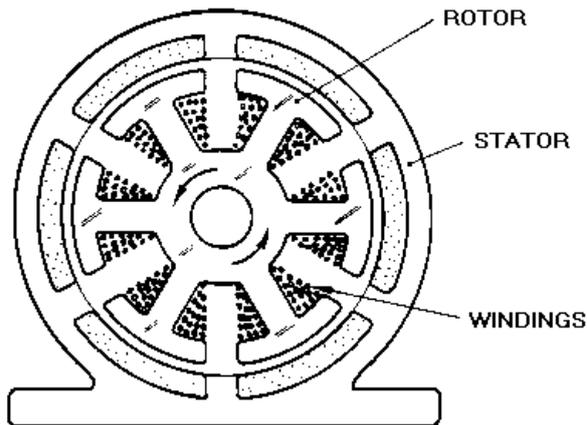
Figure 5-1. An electric motor. The maximum rotational speed can be limited by the strength of conductor used for the rotor windings
