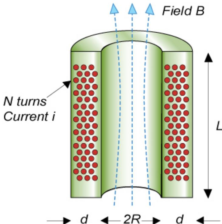
Figure 3-1. Schematic of the high-field magnet
