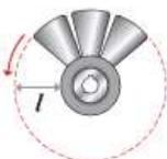
The centrifugal load on turbine blades will be one critical factor in selecting the material. The blades also must not fail due to bending during sudden turbine acceleration or to vibrations. This requires high strength and resistance to brittle failure. The blade length,  $l$ , is determined mainly by flow and space considerations and is therefore fixed.
