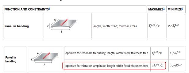
The basis of the selection is the data records for nearly 4000 engineering materials available in Level 3 of CES EduPack. These are not all candidates for the longboard deck. It is possible to put constraints in, to limit the number of materials. These constraints are based largely on the existing decks above.
