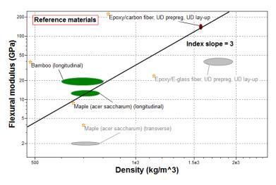
What would the effect of laminating the maple, or sandwiching these between composite layers? This can be investigated using the synthesizer tool, available in the Sustainability database of CES EduPack.
