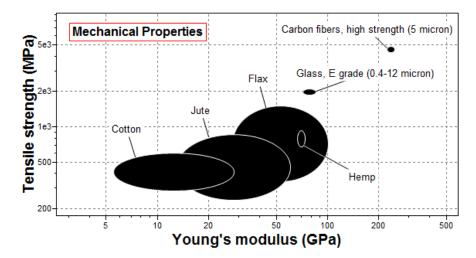
The tensile strength and stiffness for some common fibers are shown below. For stiffness, natural fibers are competitive with glass fiber, but not with carbon fiber. flax is, potentially, better than hemp both for stiffness and strength. The synthesizer can be used to estimate properties for Simple bounds composites based on Unidirectional flax fibers in a matrix of epoxy.
