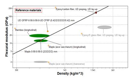
Neither lamination nor sandwiching maple multilayers between FRP face sheets improves the Material index much compared to bamboo. To improve on the performance of the bamboo skateboard deck, it is necessary to increase the bending stiffness and/or reduce the density. Any proposed structures can then be tested using the Synthesizer tool before building prototypes. This can be done (see below) in combination with improving damping properties.
