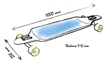
A longboard is a type of skateboard designed for downhill and slalom racing but also for simple cruising and transport. Because it is longer than a regular skateboard and normally has bigger wheels, it promotes higher speeds. Their greater weight and bulk makes them less suitable for many skateboarding tricks but contributes to stability and a fluid motion by providing more momentum.
