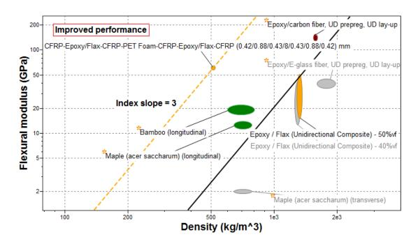
The resulting chart shows that the proposed 7-layer structure, with PET foam as the core material and the composite sandwiches as face sheets, provides a significant increase in performance. Further simulations, FE-calculations etc. are necessary but, the investigation using the synthesizer tool has provided guidance and can therefore reduce time, cost and effort in the development.
