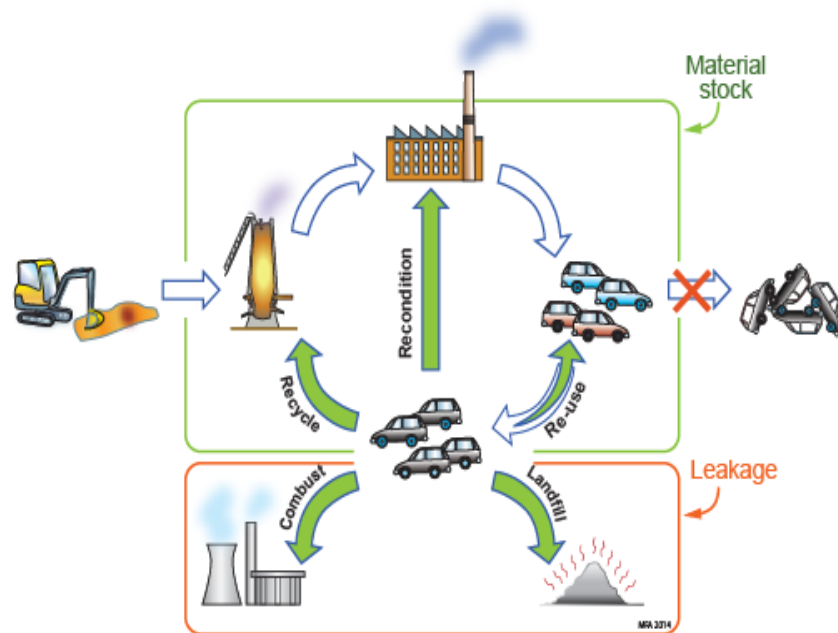
Figure 11 The circular economy. The aim is to retain materials in the “Material stock” box by reuse, reconditioning and recycling, minimizing leakage into the Waste box.
