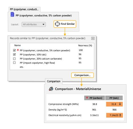
The **Comparison Table** is highlighted where there is a difference between the original (reference) and alternative materials. The reference material in this exercise was chosen specifically because it has low electrical resistivity. However, the nearest match does not, because the default criteria for nearness in this table do not account for electrical resistivity. You can change this manually.
