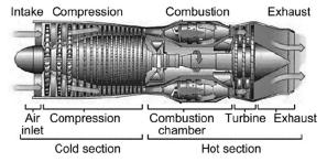
All these technologies involve challenges to the design and material choices of turbine blades. Huge tensile loads result from the centrifugal forces in addition to vibrational and bending loads. Thermal shock and creep are also issues. Nickel-based or Cobalt-based superalloys are therefore generally used for turbine parts. These retain high strength values even at high temperatures.
