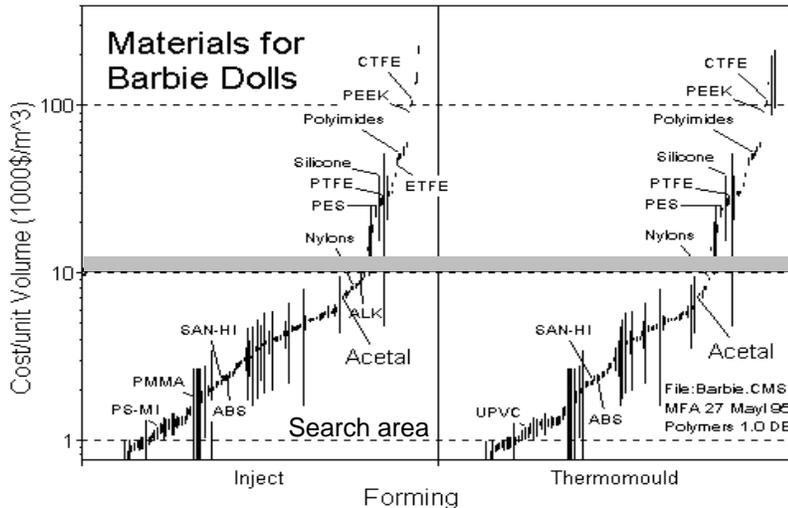
Fig 3 A bar-chart of cost against forming, using the Polymers database.
