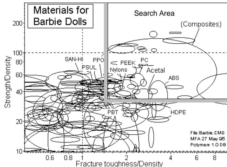
Fig 2 Chart of  $M_1$  vs  $M_2$  using the polymers database
