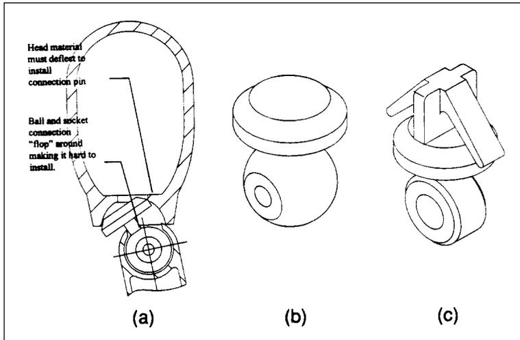
Fig 1 (a) the original neck connector design; (b) the difficulty of inserting the original connector (c) the current design
